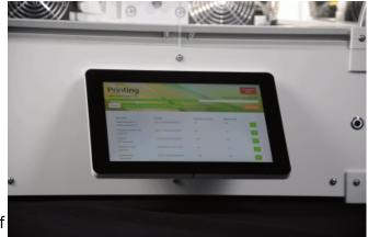
The high-resolution 10"-TFT touchscreen mounted at the front panel enables direct operation of the HT500.2.
