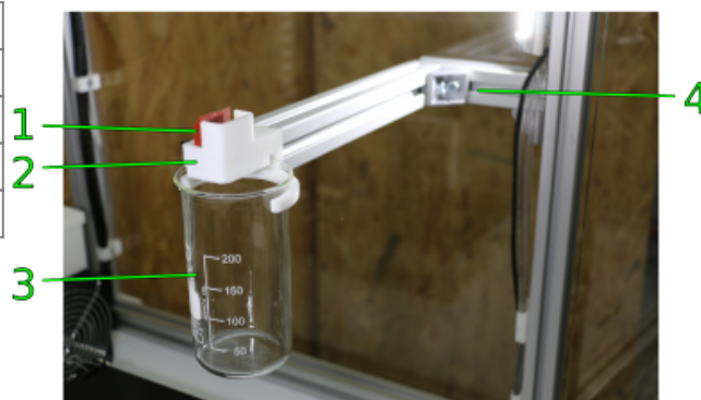
The wiper makes sure that the nozzle tip is always clean and well filled after a tool change during dual-material print jobs.
