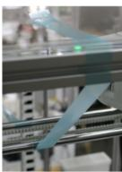
Transport restraint of the Y-axis: blue tape spans from the hind Y-shaft to the left Z-shaft and from
