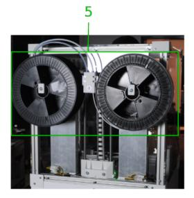
Filament supply unit at the rear side of the build chamber.
