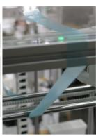
Transport restraint of the Y-axis: blue tape spans from the hind Y-shaft to the left Z-shaft and from the front Y-shaft to the top cover.
