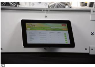
The high-resolution 10"-TFT touchscreen mounted at the front panel enables direct operation of the HT500.2.
