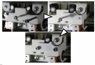
Installing the adapter for flexible filaments.
