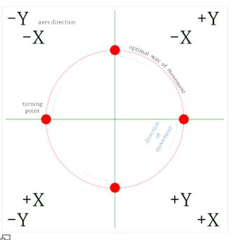
The four directions of movement and the turning points during printing a circle.
