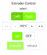
This new feature was installed to give you the opportunity of finding the correct extrusion temperature of any material more directly and comfortably without having to use the [Prime Extruders] wizard.
