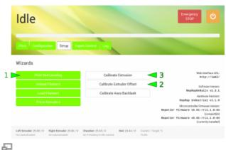
Leveling and offset calibration are done via the GUI. Both only needs to be done once if no hardware changes are performed.
