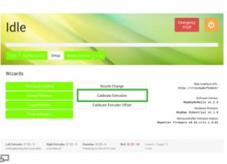
Choose the [Calibrate Extrusion] wizard from the *Setup* menu (either software version).
