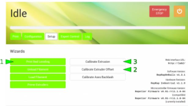
Leveling and offset calibration are done via the GUI. Both only needs to be done once if no hardware changes are performed.
