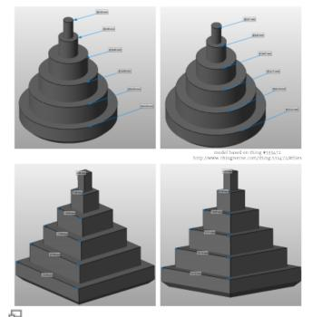
netfabb visualization of the ABS test bodies printed for comparison and evaluation. On the left hand-side the uncompensated model, on the right-hand side the model after multiplying with  $\alpha_1$  prior to exporting the .stl.
