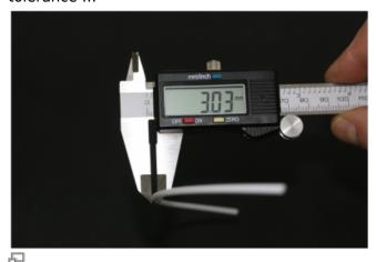
Measured at the same position, turned 90°. The diameter now exceeds the tolerance - the filament is out of round and must be replaced.
