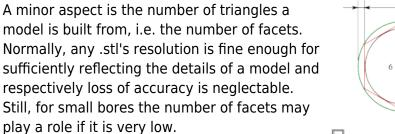
The graphic on the right displays the possible influence of facets on an inner diameter. In case of roughly faceted objects try increasing the resolution of your CAD model to improve dimensional accuracy.
