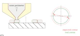
Overfilling of the inside of the extrusion strand reduces the diameter of small holes.
