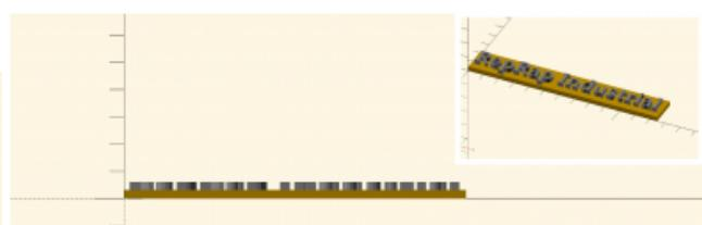
3D model preparation for bicolored printing example 2: both individual parts of the 3D model being aligned in a common assembly and exported as separate STL-files with the correct relative coordinates.
