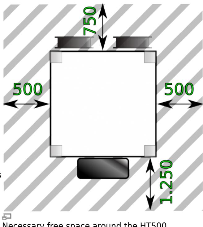
air circulation at the ventilation grill in the back cover. At the front a free space of 1.250mm is recommended to allow easy operation with open chamber doors.
