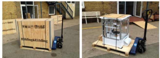
The wooden box and the lid are fastened to the pallet with tensioning straps. The 3D Printer is padded with air cushion foil and a wooden cover plate and strapped to the pallet with tensioning straps.
