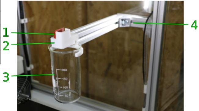
The wiper makes sure that the nozzle tip is always clean and well filled after a tool change during dual-material print jobs.
