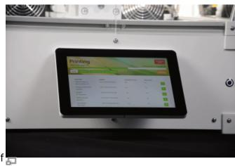
The high-resolution 10"-TFT touchscreen mounted at the front panel enables direct operation of the HT500.
