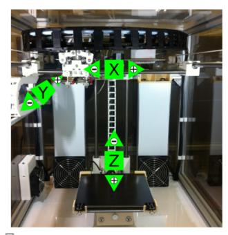
Denotation and direction determination of the axes.
