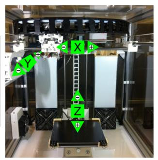
Denotation and direction determination of the axes.
