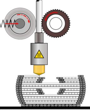
The layer-by-layer build-up of random geometries becomes possible with FFF-3D Printers.
