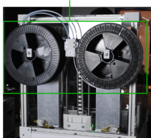
Filament supply unit at the rear side of the build chamber.
