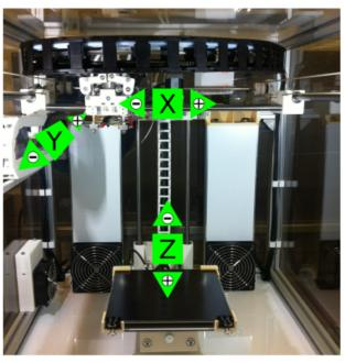
Denotation and direction determination of the axes.
