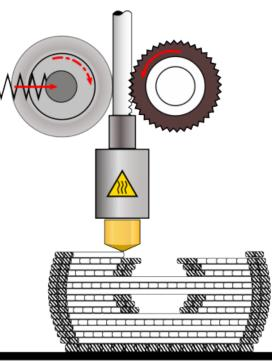
The layer-by-layer build-up of random geometries becomes possible with FFF-3D Printers.
