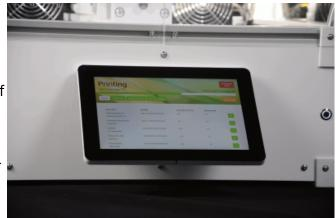
The high-resolution 10"-TFT touchscreen mounted at the front panel enables direct operation of the HT500.
