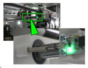
Hall effect sensor and magnet of the X-axis.
