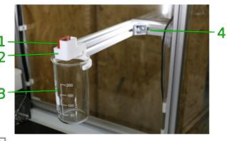
The wiper makes sure that the nozzle tip is always clean and well filled after a tool change
