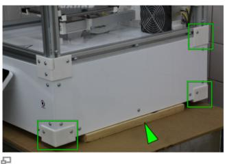
Lift the 3D Printer at one side; the feet and the hind cover angle must be removed.
