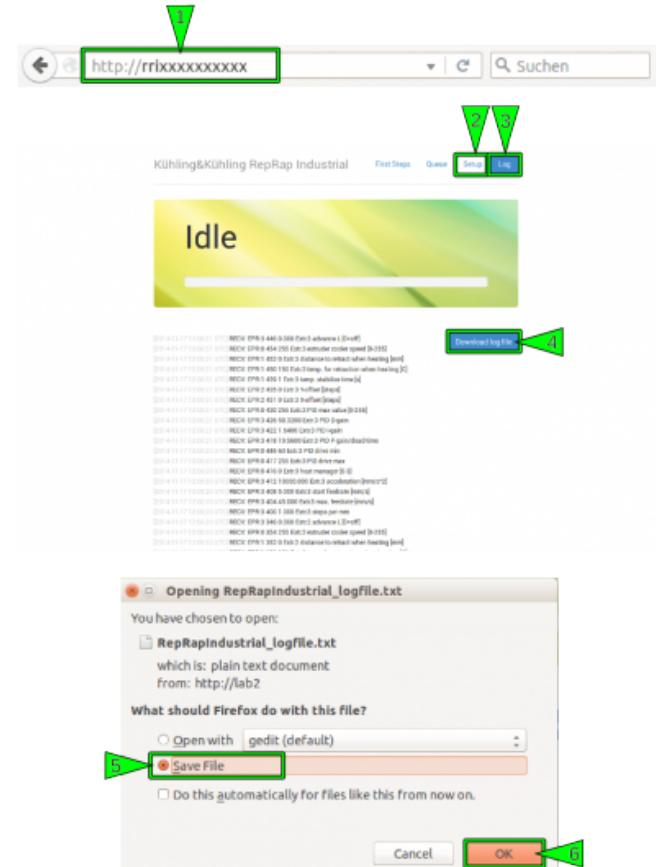
Downloading the log files via the web interface (same procedure for software versions v1.0.5 and v1.1.0). Please remember opening the *Setup* tab first.
