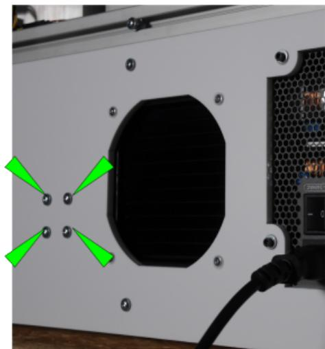
☞ Holding screws of cooling water pump.
