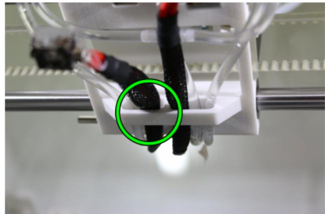
Make sure that the cables are correctly guided through the lead-through during re-installation.
