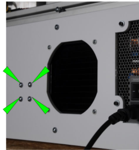
Holding screws of cooling water pump.
