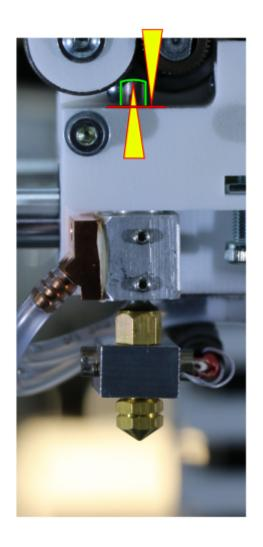
Barrel pushed up too far into its seat (exaggerated).
