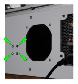
Holding screws of cooling water pump.
