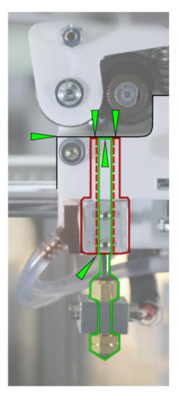
Aligning the extruder barrel and the hot end mount's upper rim.
