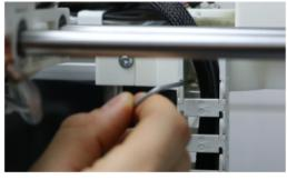
Use the #2 Allen key to loosen the set screw.
