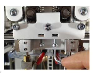
Adjusting the idler lever preload.
