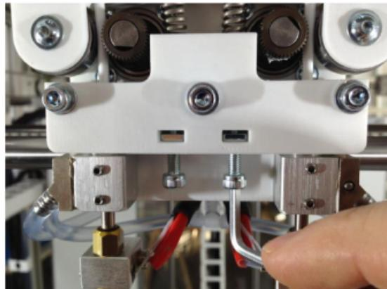
Adjusting the idler lever preload.
