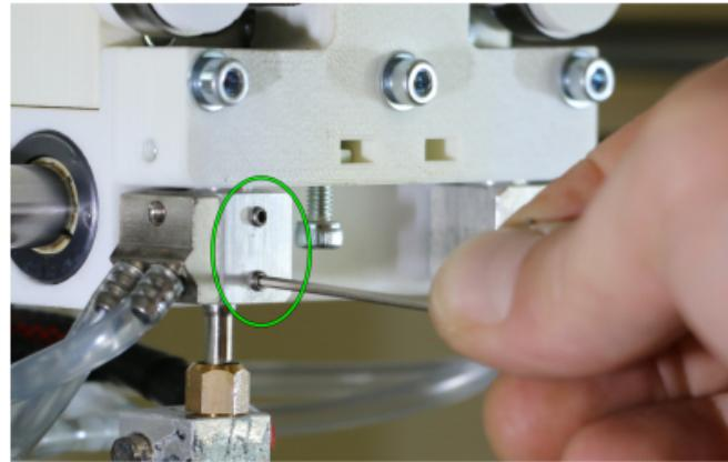
Loosening the hot-end mount set screws is mandatory to avoid breaking the glued connection of barrel and melter.
