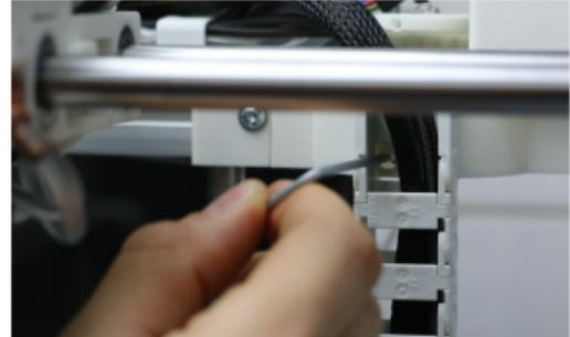
Use the #2 Allen key to loosen the set screw.
