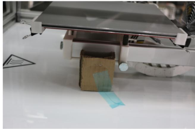
Place the cardboard support underneath the print table and fix it with tape.
