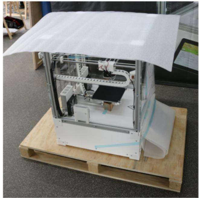
Place the 3D Printer in the middle of the pallet and cover it with foam foil.
