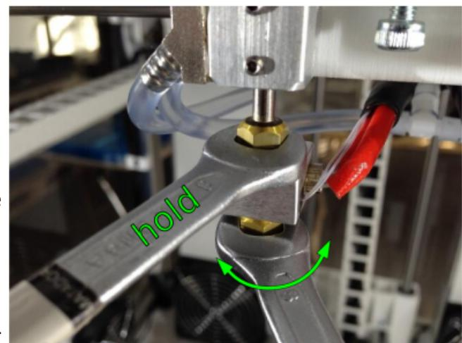
Unscrewing and fastening the nozzle tip requires attention not to overwind and sheer off the thread.
