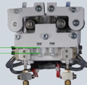
Too high tension of the idler lever spring may result in the gear drive to slip and grind into the filament. Too low tension of the idler lever spring may result in slipping of the gear drive. In both cases the print will abort due to insufficient material transport.
