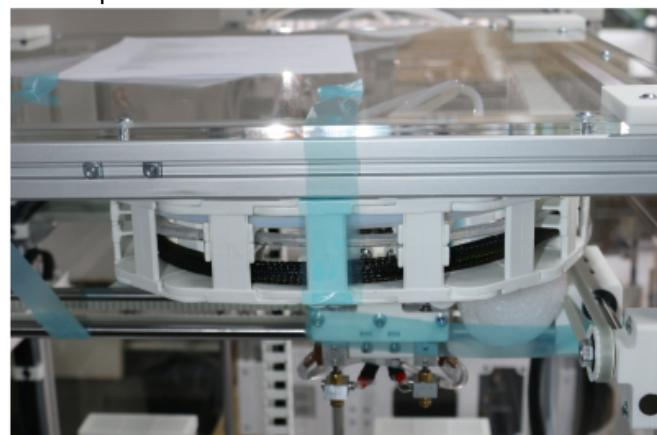
Entwine the e-chain with tape and fasten it to the printer's top cover.
