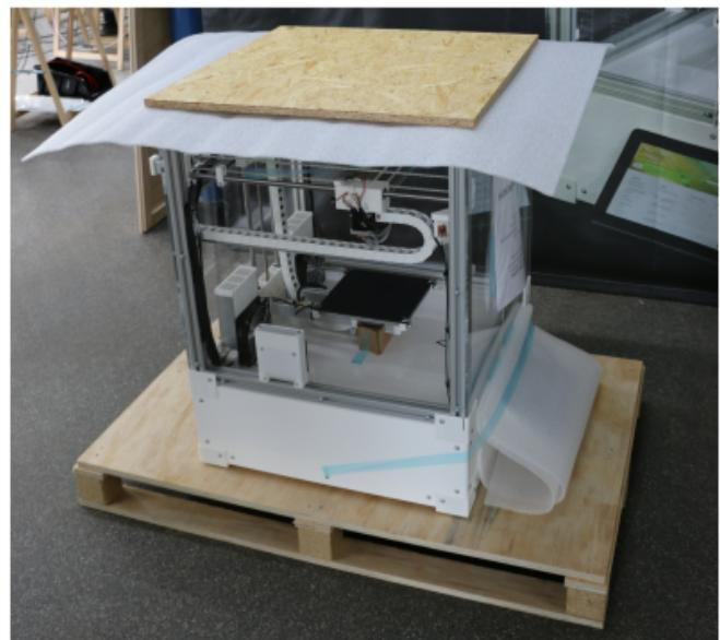
The cover plate protects the printer when strapping it down.
