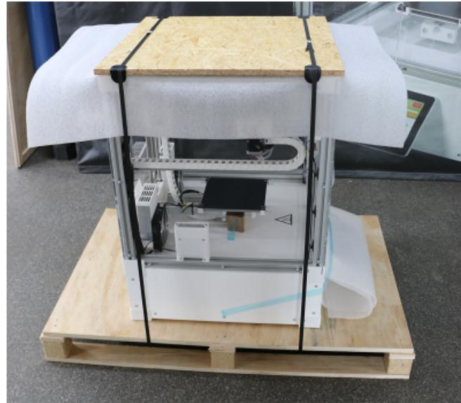
☞ The 3D Printer must be tightly secured on the transport pallet.
