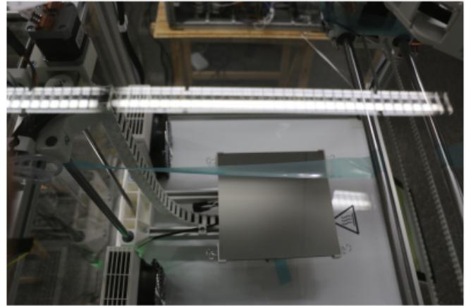
Entwine the hind shaft of the H-bridge with tape and fasten it to on of the Z-axes.
