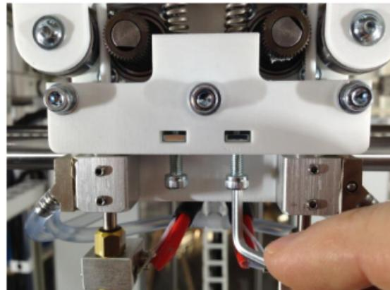
Adjusting the idler lever preload.
