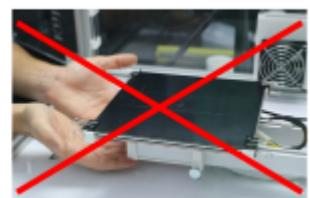
To test if the clamp collar has come loose, **carefully** try to lift the print table and observe the Z-drive pulley.
