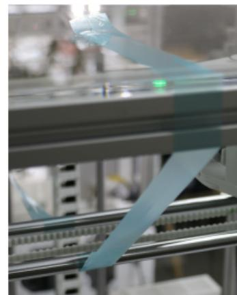
Entwine the frontal shaft of the H-bridge with tape and fasten it to the printer's top cover.
