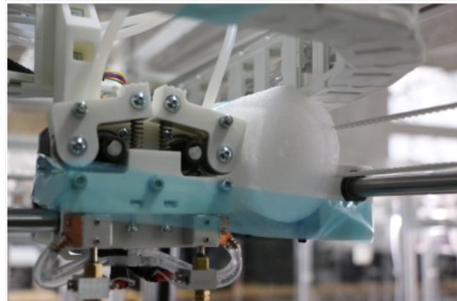
Cushion the extruder head with the foam coil against the right carriage and tightly fasten it with tape.
