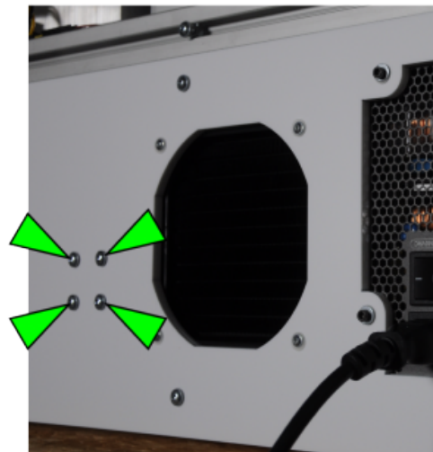
Holding screws of cooling water pump at the rear cover of the electronic chamber.
