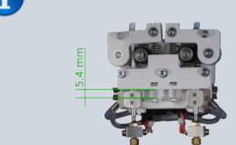
Too high tension of the idler lever spring may result in the gear drive to slip and grind into the filament. Too low tension of the idler lever spring may result in slipping of the gear drive. In both cases the print will abort due to insufficient material transport.
