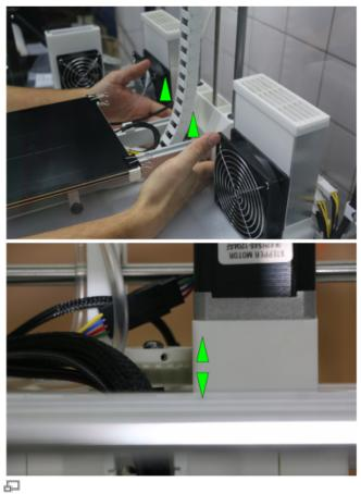
Try to lift the Z-elevator and watch the pulley. If the pulley moves up and down, the clamp collar must be repositioned.
