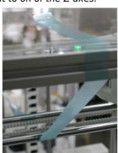
Entwine the frontal shaft of the H-bridge with tape and fasten it to the printer's top cover.
