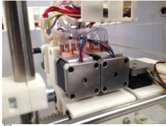
Dual extruders, back view - water cooled planetary geared stepper motors
