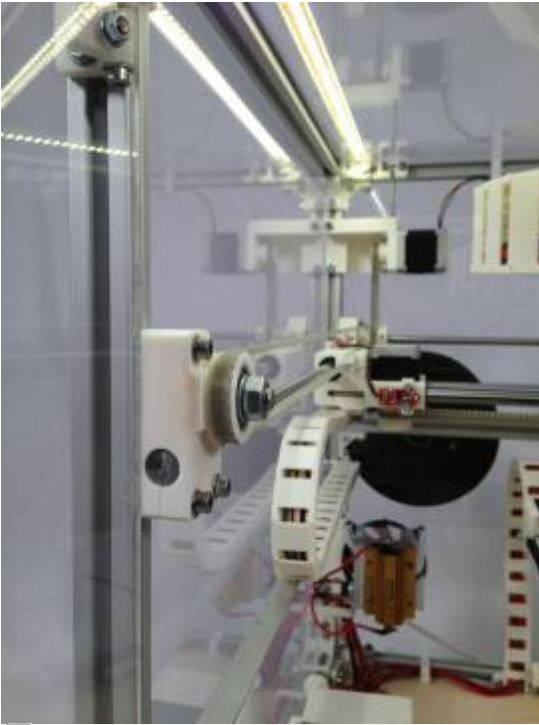
Front left Y end with belt idler
