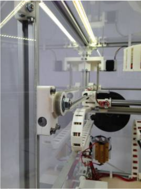
Front left Y end with belt idler
