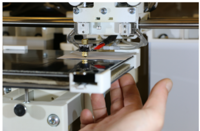
Manual leveling with paper spacer - front and hind right leveling point.
