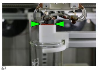
Nozzle cone and wiper lip are correctly aligned.
