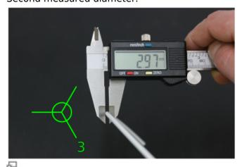
Third measured diameter - this filament exceeds the stated tolerance and must be replaced.
