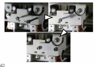
Installing the adapter for flexible filaments.
