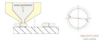
Overfilling of the inside of the extrusion strand reduces the diameter of small holes.
