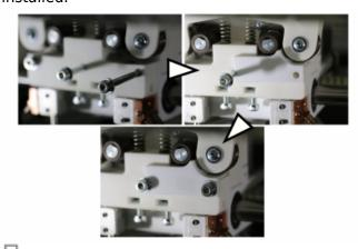
Installing the adapter for flexible filaments.
