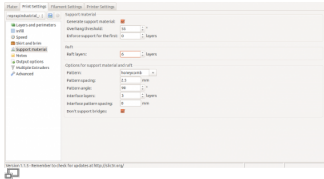
Slic3r Print Settings - adding raft layers
