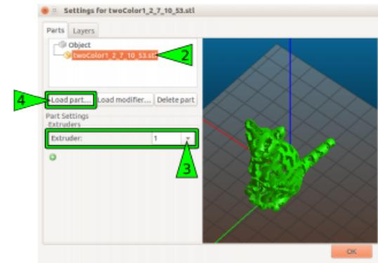
After the extruder for the first part has been assigned, the second part is loaded via the *Settings* dialog.
