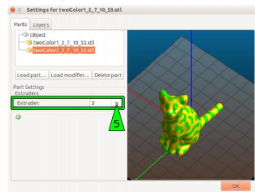
The second part must be assigned to extruder 2.
