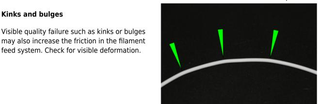
Visible kinks in the filament may also lead to jamming.
