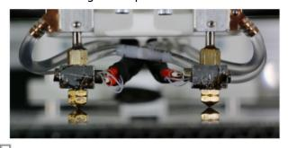
Precise leveling of both hot ends is mandatory for dual extruder prints.
