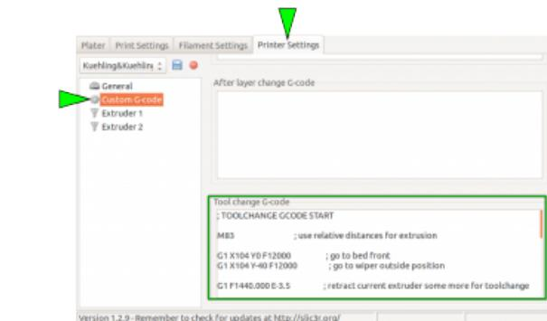
The Slic3r tool change G-code provides the information for the wiping process. It is preconfigured and normally does not need interference.
