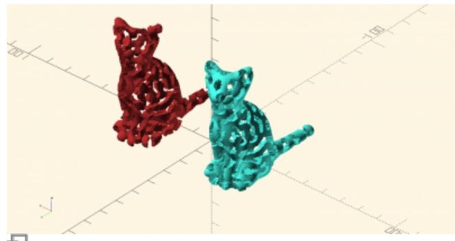
3D model preparation for bicolored printing example 1: a model (<http://www.thingiverse.com/thing:62536>) split in two for bicolored printing. Both must be aligned with the same relative position and exported as separate STLs.
