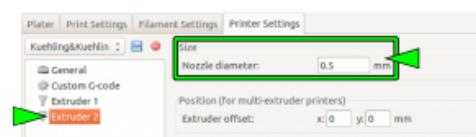
Make sure the correct nozzle size has been entered for each extruder.
