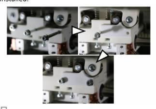
Installing the adapter for flexible filaments.
