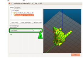
The second part must be assigned to extruder 2.
