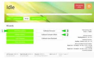
Leveling and offset calibration are done via the GUI. Both only needs to be done once if no hardware changes are performed.
