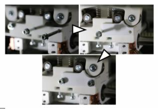
Installing the adapter for flexible filaments.
