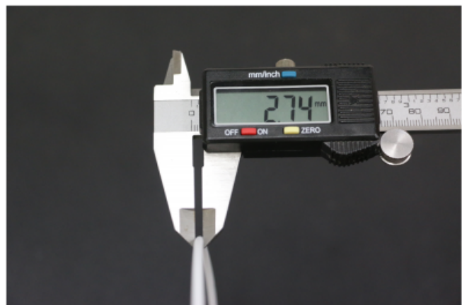
The measured diameter is below the admissible tolerance ...
