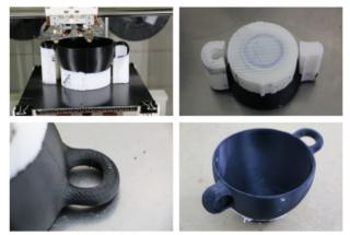
Excavation finding of the Archeological Institute Things no. 67503 and 318057 from of the University of Freiburg, reprinted on a RepRap Industrial with black ABS and HIPS as soluble support.
