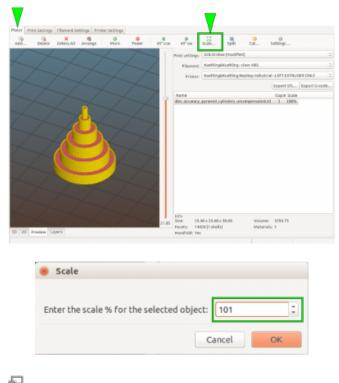
Scaling the model directly in Slic3r.
