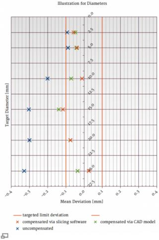
The deviation decreases significantly when the thermal expansion is compensated.
