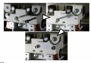
Installing the adapter for flexible filaments.
