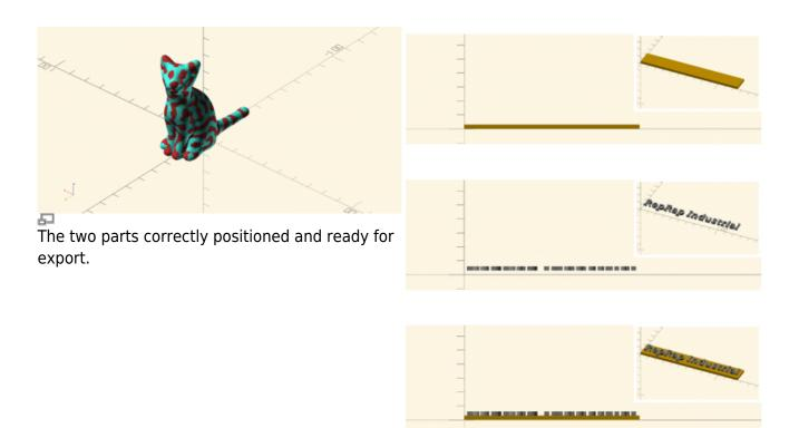
3D model preparation for bicolored printing example 2: both individual parts of the 3D model being aligned in a common assembly and exported as separate STL-files with the correct relative coordinates.
