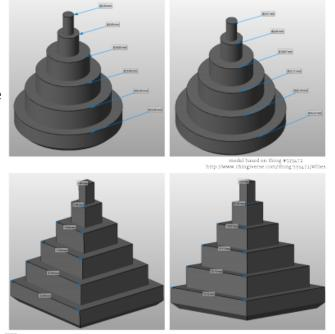
netfabb visualization of the ABS test bodies printed for comparison and evaluation. On the left hand-side the uncompensated model, on the right-hand side the model after multiplying with
