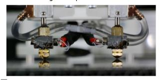
Precise leveling of both hot ends is mandatory for dual extruder prints.
