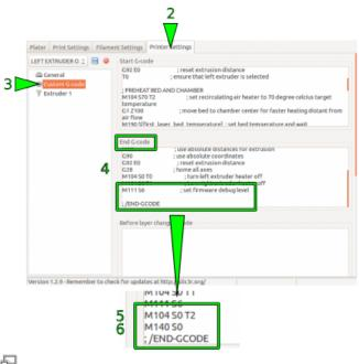
Switching off the build chamber heating
