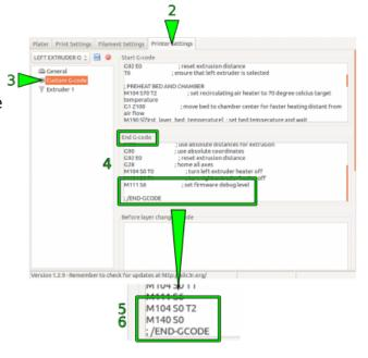
Switching off the build chamber heating elements by modifying the Slic3r custom End G-code.
