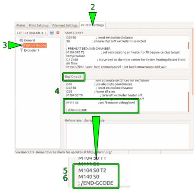
Switching off the build chamber heating elements by modifying the Slic3r custom End G-
