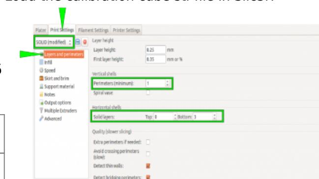
Select the *Layers and perimeters* according to the adjacent table.
