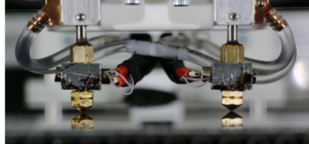
Precise leveling of both hot ends is mandatory for dual extruder prints.
