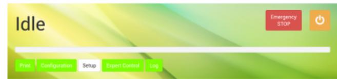
Choose the [Calibrate Extrusion] wizard from the *Setup* menu (either software version).
