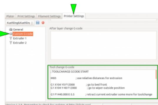
All necessary settings to effect the required movement of the print head into a g-code are implemented in the Tool change G-code in the Custom G-code menu of Slic3r's *Printer Settings*. It is only filled in when one of the [Dual Extruder](#) profiles has been chosen.
