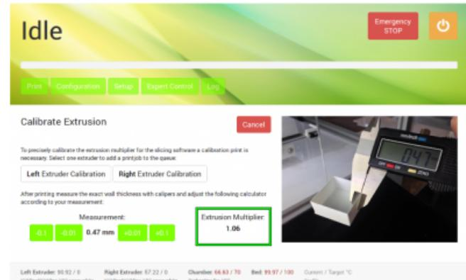
Adjust the preset “0.50 mm” value via the touch buttons and read the necessary extrusion multiplier directly from the display.
