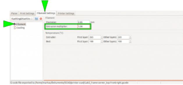
Enter the extrusion multiplier in Slic3r and save the filament profile (rename!).
