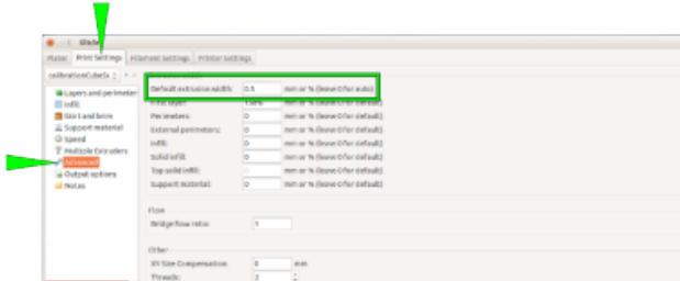
Select the *Default extrusion width* according to the adjacent table.
