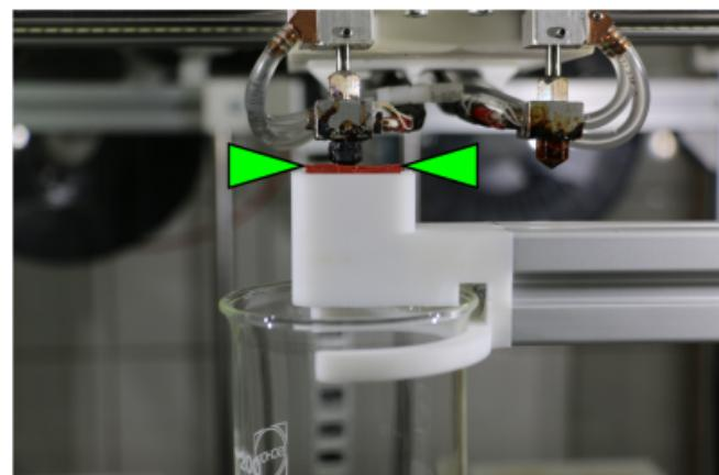
Nozzle cone and wiper lip are correctly aligned.
