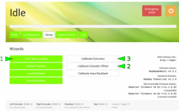
Leveling and offset calibration are done via the GUI. Both only needs to be done once if no hardware changes are performed.
