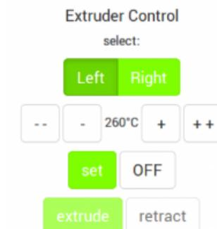
Try finding the suitable temperature by directly extruding via the [Expert Control](#) screen.
