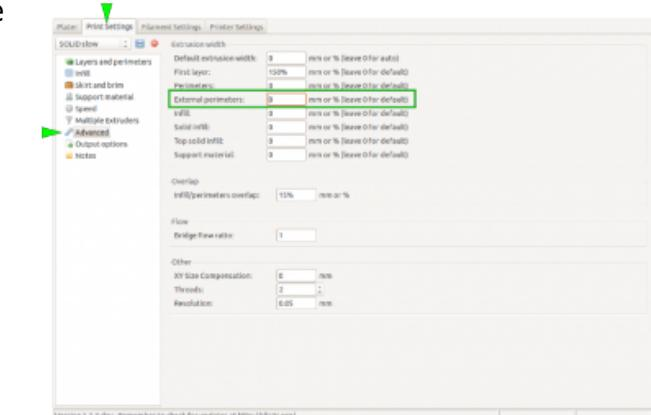
Reducing the outer perimeter extrusion width in Slic3r.
