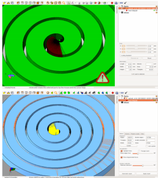
Alert of mismatches in an STL and the preview of misaligned edges and holes in netfabb basic's part repair.
