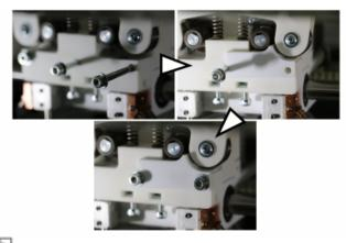
Installing the adapter for flexible filaments.
