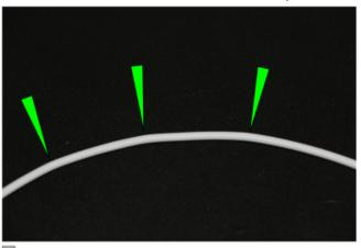
Visible kinks in the filament may also lead to jamming.
