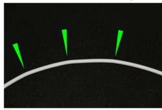
Visible kinks in the filament may also lead to jamming.
