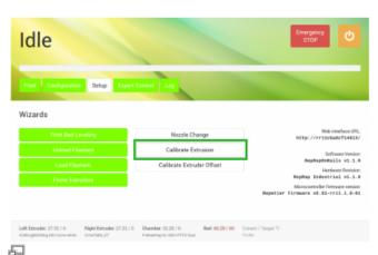
Choose the [Calibrate Extrusion] wizard from the *Setup* menu (either software version).
