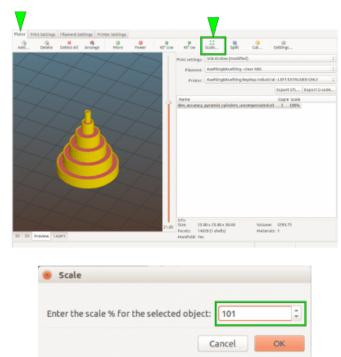
Scaling the model directly in Slic3r.
