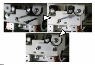
Installing the adapter for flexible filaments.
