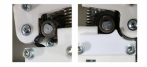
Flexible filament bending and twisting without and extruding smoothly with the adapter installed.
