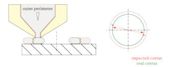
Solution of the inside of the extrusion strand reduces the diameter of small holes.
