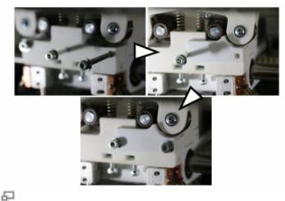
Installing the adapter for flexible filaments.
