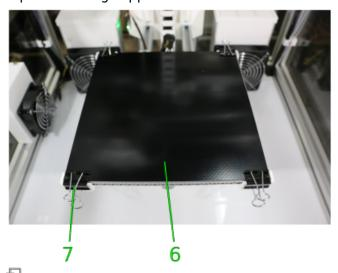
Print bed fastened with four bulldog clamps (hardware revision 1.1.0).
