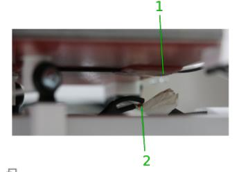
Thermistors of the print bed (1) and the build chamber (2).
