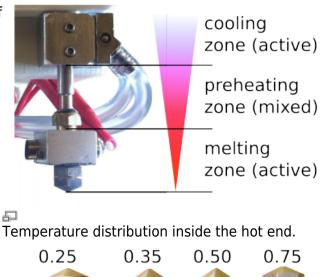
The nozzle is exchangeable to provide different bore diameters for different materials, layer thicknesses or print speed. Ex factory, the 0.35 mm tip is preinstalled. Additionally, three nozzle tips with diameters of 0.25 mm, 0.5 mm and
