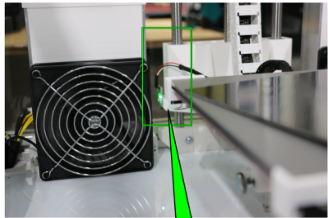
Hall effect sensor and magnet of the Y-axis.
