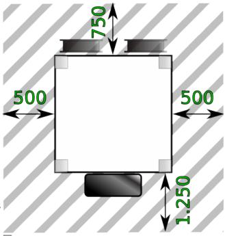
to make changing the material easy and to ensure free air circulation at the ventilation grill in the back cover. At the front a free space of 1.250mm is recommended to allow easy operation with open chamber doors.
