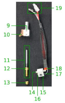
Hot end disassembled
