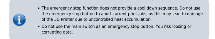
When the Emergency Stop is triggered, the microcontroller board responsible for the stepper motors, heaters and sensors is reset immediately and returns to idle state afterwards. Now it is safe to resolve any problems or defects in the build chamber. The build chamber can then be reactivated via the *Manual Control* screen or by starting a print job as usual.
