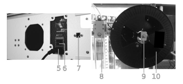
Power/network connections and mains switch at Filament feed system at the rear of the build the rear panel.
