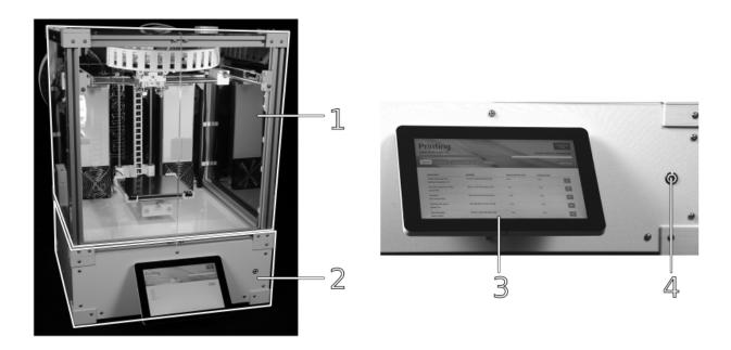
The two main functional sections of the RepRap HMI touchscreen for direct operation and wake Industrial 3D printer: the build chamber with the button at the front panel. functional components and the electronic
