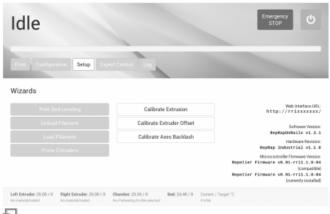
The web-interface URL on the SETUP screen is required for connecting the 3D printer with your local network.
