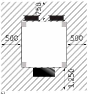
Network Time Protocol (ntp). Free space required for optimal operation of the Refer to the online manual if your network RepRap Industrial 3D Printer.
