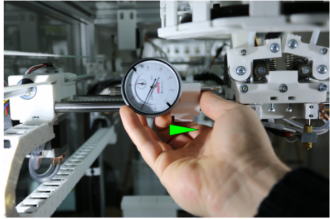
Installing the dial gage at the X-axis.
