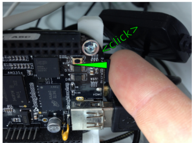
“Push and release” the SD card.
