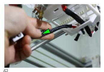
Pull the cable through the lead-through and remove the heating block.
