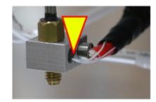
• Loosen the set screw again and pull the barrel out of the seat.
