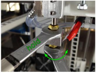
Unscrewing and fastening the nozzle tip requires attention not to overwinde and sheer off the thread.
